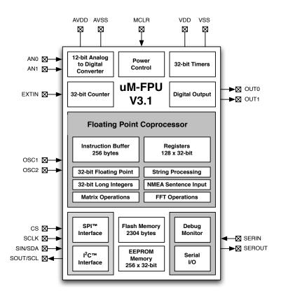
The uM-FPU V3.1 chip easily interfaces to virtually any microcontroller using an SPI<sup>m</sup> or I<sup>2</sup>C<sup>m</sup> interface.
